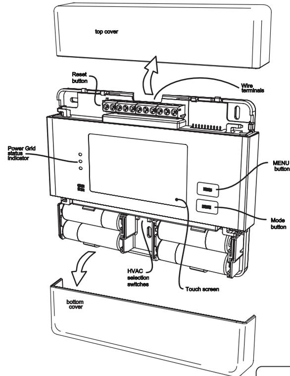
**Statement of use:** 100% Compatible with all popular residential HVAC systems; 24VAC single, two stage conventional heating systems (gas/oil/electric), heat pumps with up to two stages of heat and two stage auxiliary heat (electric or fossil), zoned forced air and zoned hot water (2 or 3 wire), millivolt systems (with a 12-24 AC or DC source), one or two stage cooling, and hybrid systems.
